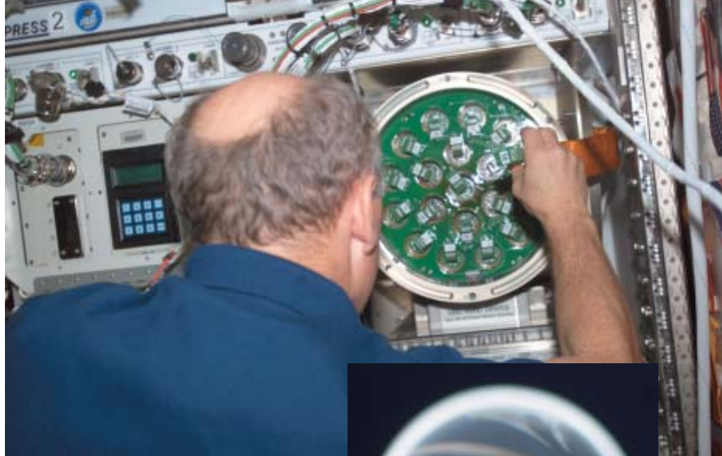
Kenneth Bowersox, Expedition Six mission commander, inserts an experiment cartridge in the autoclave for the Zeolite Crystal Growth (ZCG) experiment in Destiny, and (inset) view of a bubble formed as a result of the experiment.
