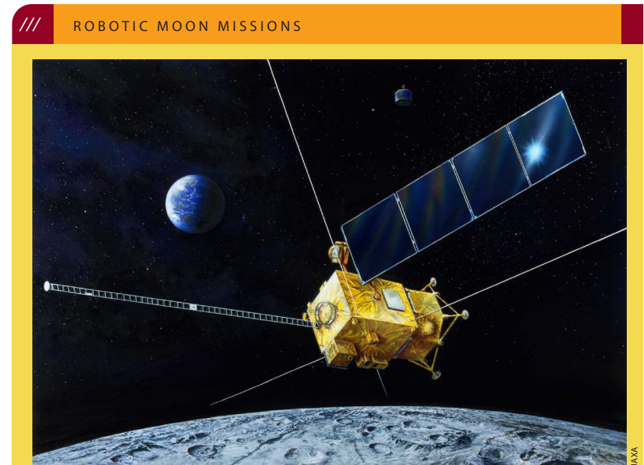
AFTER ORBITING THE MOON for a year, the Selene probe will detach its propulsion module, which will make an automated soft landing on the Moon.
