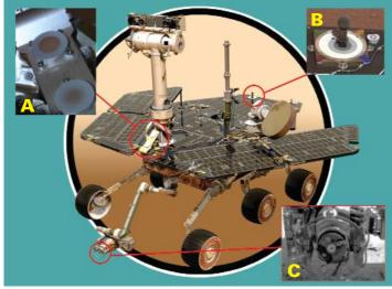
Details: (A) dust collection magnets, (B) color calibration sheets with sundial (provided by Planetary Society) and (C) rock abrasion tool.
