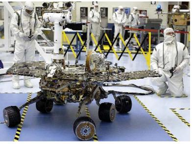
The Mars Exploration Rover has six wheels, each with its own individual motor. the two front and two rear wheels also have individual steering motors (1 each). These Rovers can turn a full 360 degrees in place, and can swerve and curve while driving.
