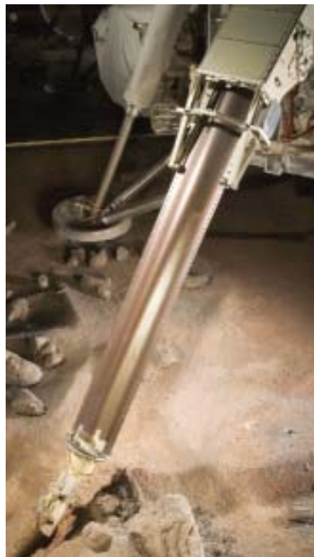
Detail of the Viking robot arm. It was compressed and rolled up inside the deployment box, and then assumed its cylinder shape as it was extended.
