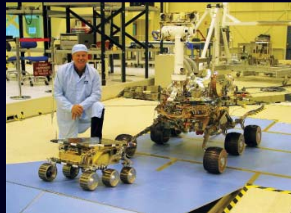
Potpourri of early NASA Mars Rover designs, leading to the Sojourner mini-rover deployed by the Pathfinder lander in 1997. Left—the Sojourner (and human friend) next to its direct descendant, the much larger (and long-lived) Spirit and Opportunity class of rover.
