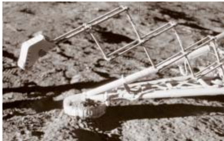
This Surveyor moon robot arm (scissors design) was photographed by Apollo astronauts, who visited it in 1969.
