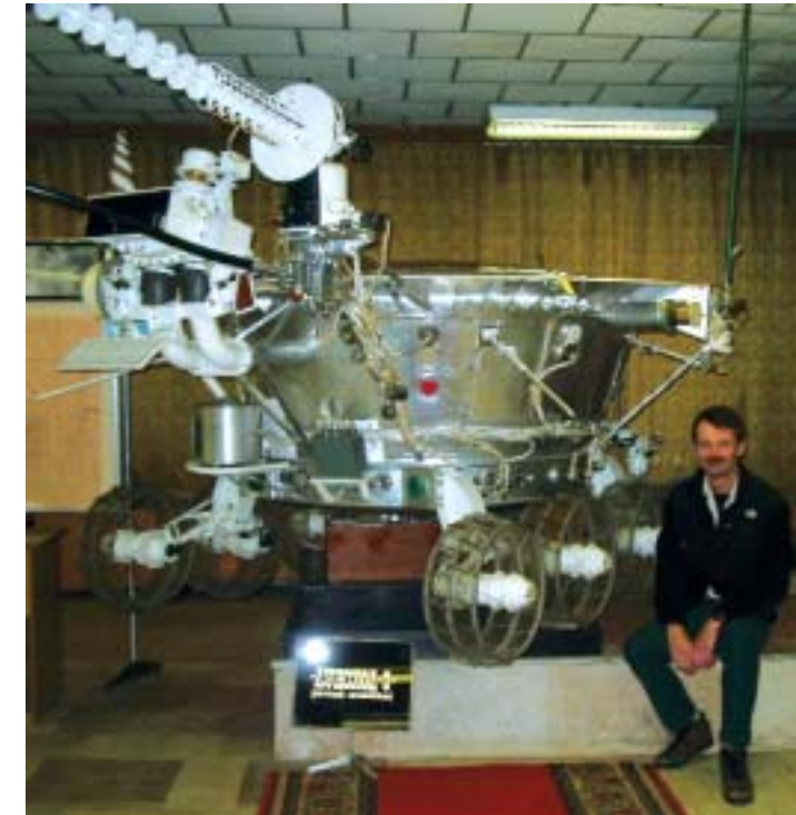
Seven-wheeled Soviet 'Lunokhod' moon rover, a backup unit to two rovers that successfully reached the moon in the early 1970s. Photo courtesy of Digby Tarvin.
