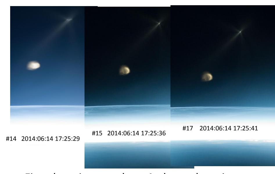
First three images show 4-plume thrusting and circular cloud behind rocket
