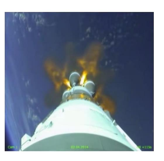
Conventional wisdom is that streamers indicate engine plumes. Recently released Soyuz ascent rocketcam videos suggest visible streamers may form at interface of two invisible engine plumes [alternately this shows plumes of core stage brighter than strapons]. Video shows stage-1.
